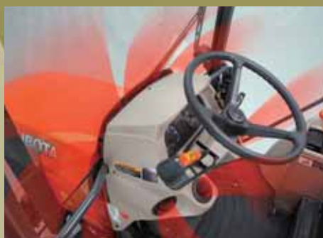
Air is circulated throughout the windshield to prevent icing, frosting and fogging.
