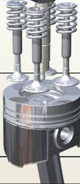
4-valve, Center-Direct Injection System
